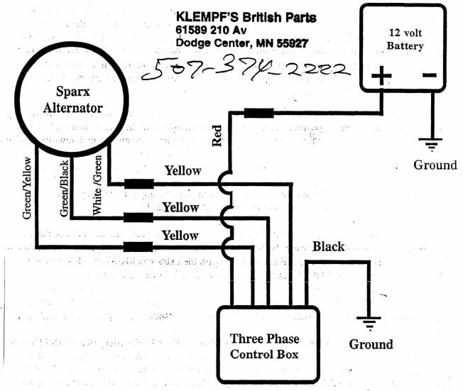
There will be no voltage output from the regulator until it is connected to a "known good" 12 volt battery. To test the output from the regulator you must have it connected to a known good battery.
