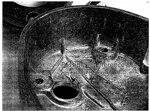
Due to manufacturing tolerances, and the increase size of the 3 phase stator, some Triumph T140s can have some interference between the Sparx stator and the primary cover. If present, the primary cover is held away from the engine cases by the thickness of a primary gasket. Careful removal of a little material on the primary cover's inner bosses (shown in photo) will cure the problem.
